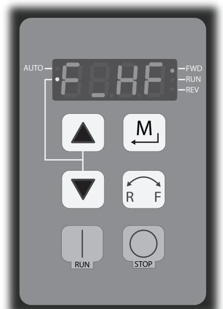
Typical fault message display (incoming line over-voltage shown)
